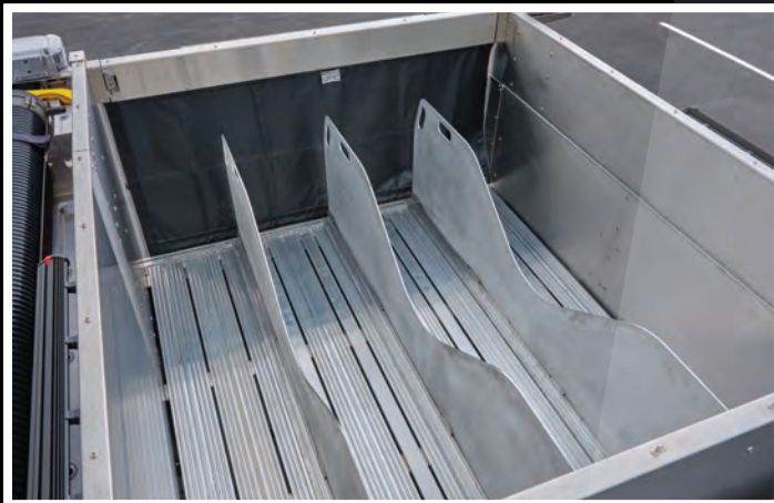
Adjustable hosebed dividers. Total hosebed capacity: 124.9 cu. ft.
