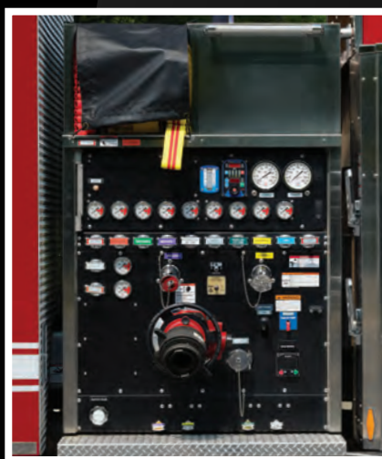
Side-Mount Pump Module (Waterous)
