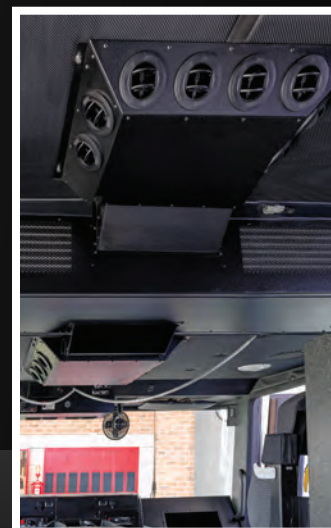
High Performance HVAC System (Output: 90,000 BTUs)
