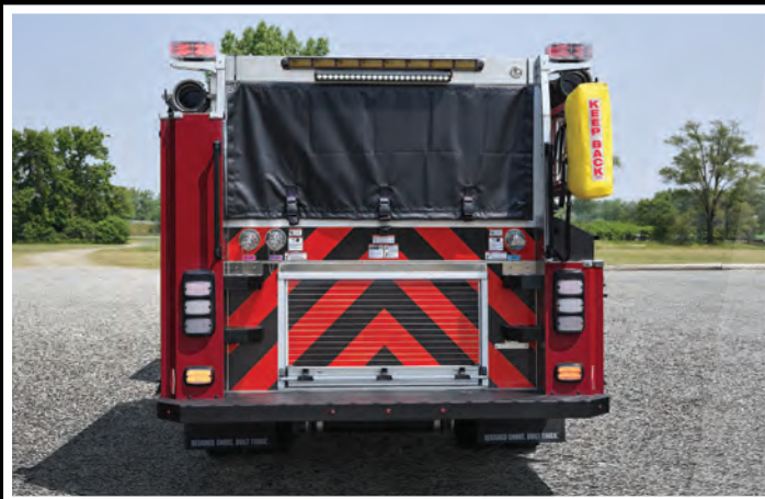
Low hosebed height (66") for easy access and safer hose loading
