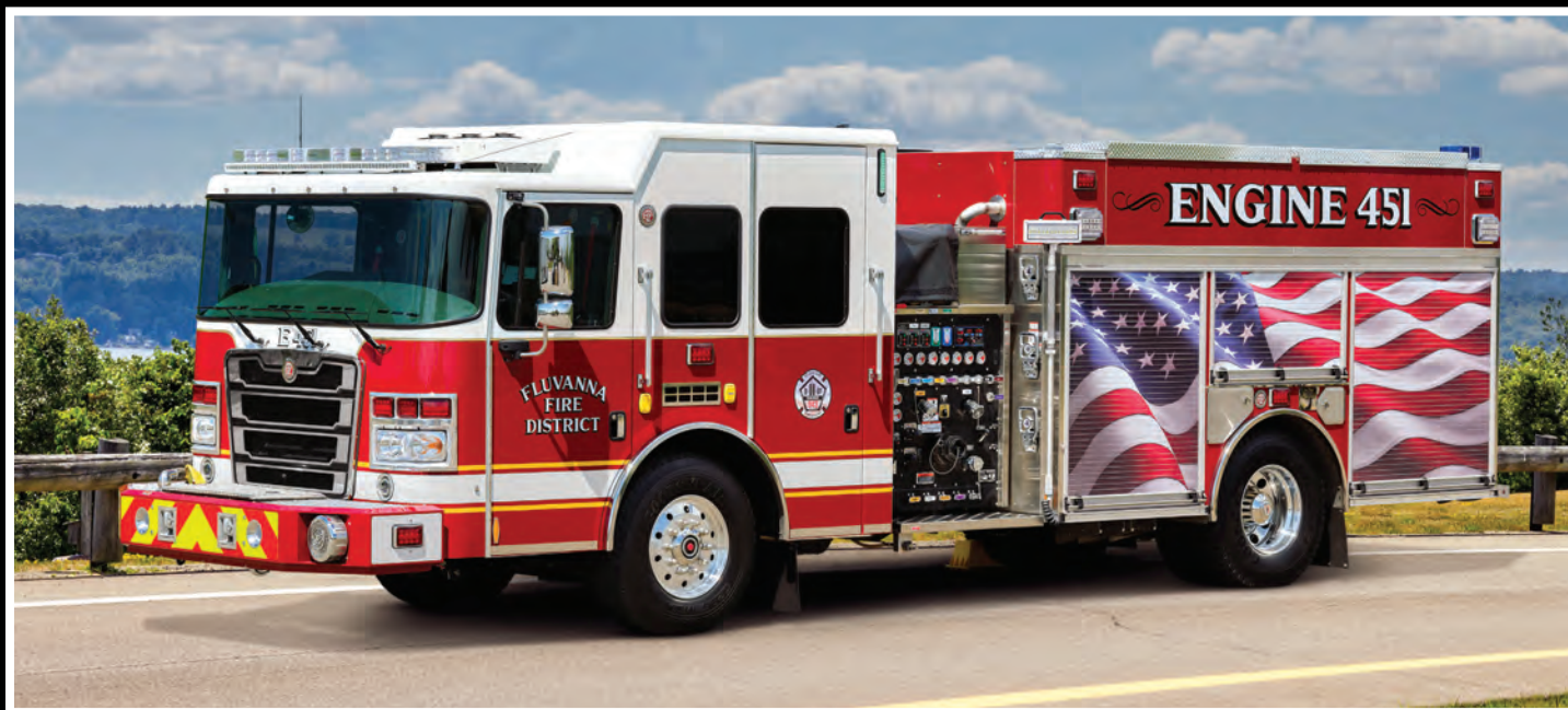
One-piece Windshield for Maximum Visibility: (3,150 sq. in.). Traditional Ladders (On the Side).
