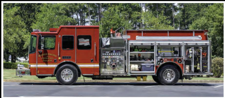
The **CORE22** on the 1871 chassis is also available without coffin compartments and hard suction stored on top.
