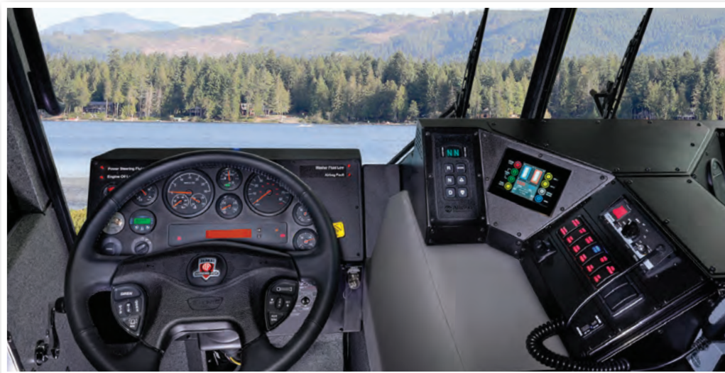
Vinyl ester composite dash and center console for durability
