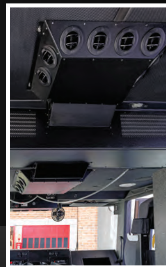
High Performance HVAC System (Output: 90,000 BTUs)
