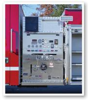
Internal ladder storage (on-beam)  Proven pump module: Hale Qmax (1500 GPM)
